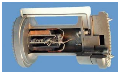
Fig. 1: Cut model of the telemeterized VBR
