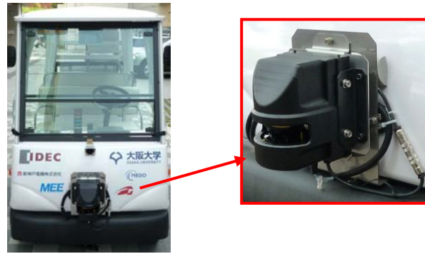
Figure 5. Safety laser scanner for outdoor use installed on the golf cart
