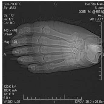
Figure 11. CT image of a bear's foot after run-over test. Trolley mass: 210kg. Traveling speed: 14km/h. Tire: Pneumatic tire inflated to 350kPa.
