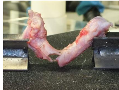
Figure 8. Load-bearing characteristics of a bear's foot bone. Figure 9. Bone fracture by bending test.
