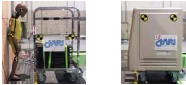
Figure 4 Left: Collision between a child dummy in front of a wall and a moving object that represents a mobile robot with a steel structure. Right: Object that represents a mobile robot with an elastic polystyrene panel.
