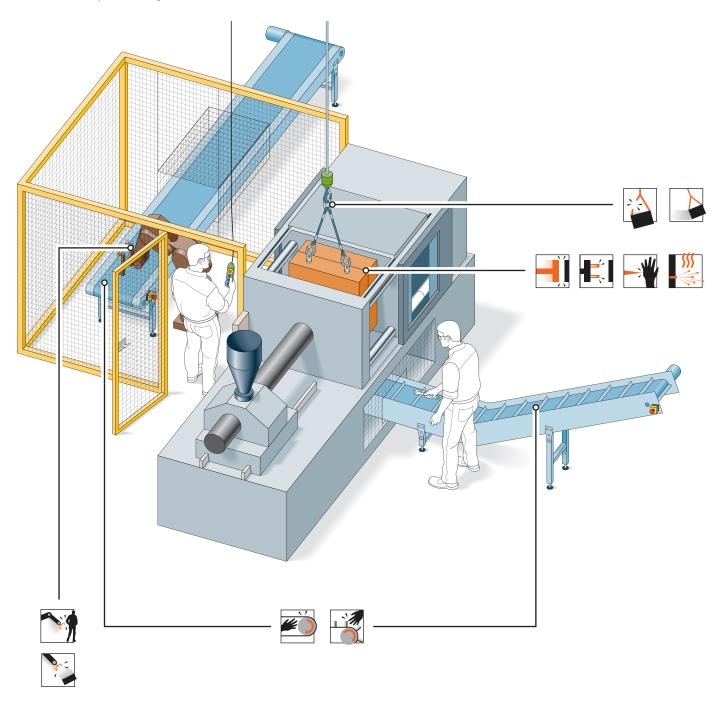
Auxiliary equipment used with injection molding machines has its own hazards. It may also generate new risks, depending on how it is integrated into the system.
