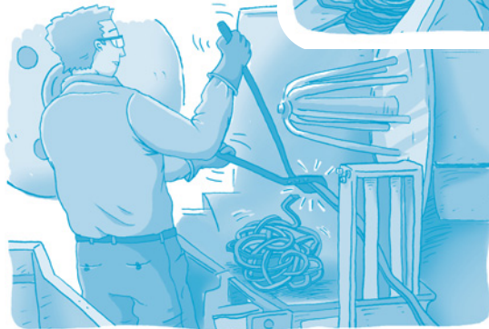
Fig. 2.6 Operator who has to cut and reattach the metal strip that has detached from the reel.
