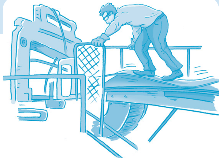
Fig. 2.2 Operator climbing on the metal sheet to insert it properly in the slitter.
