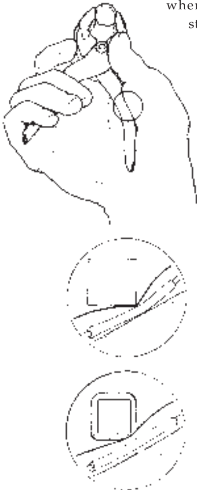
Fig. 2.18 A poorly designed grip can compress the tendons at the base of the thumb
