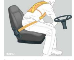
This retractor allows good body mobility and is similar to the one found in cars. The operator can shift his position on the seat to obtain better visibility when driving backwards and can lean over easily to access hard-to-reach zones (figure 1). This mechanism is therefore less likely to cause discomfort.
