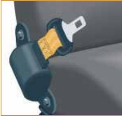
**Retractors serve to retract, or rewind, the slack webbing in seat belts into a housing drum.**
