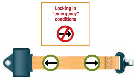
The retractor includes a number of devices (e.g. a ball-bearing system) that lock the webbing in "emergency" conditions. Given the particular locking mechanism of the ELR, it is essential to follow the manufacturer's recommendations during installation.
