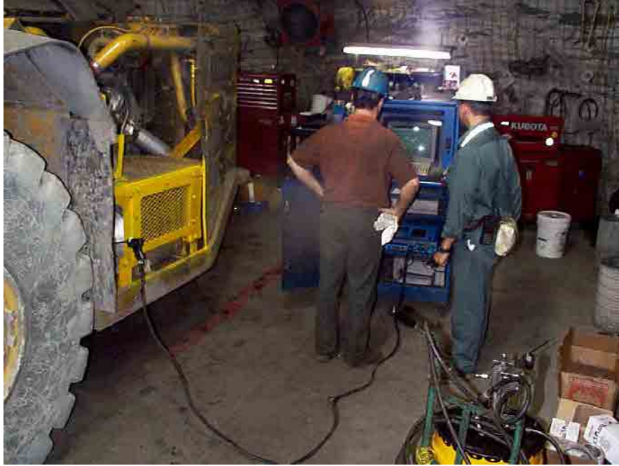
Figure 5. UGAS/ECOM Direct Exhaust Sampling
