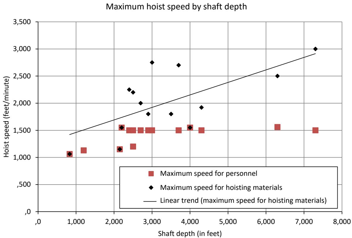
**Figure 5. Maximum speed of conveyance by shaft depth**
