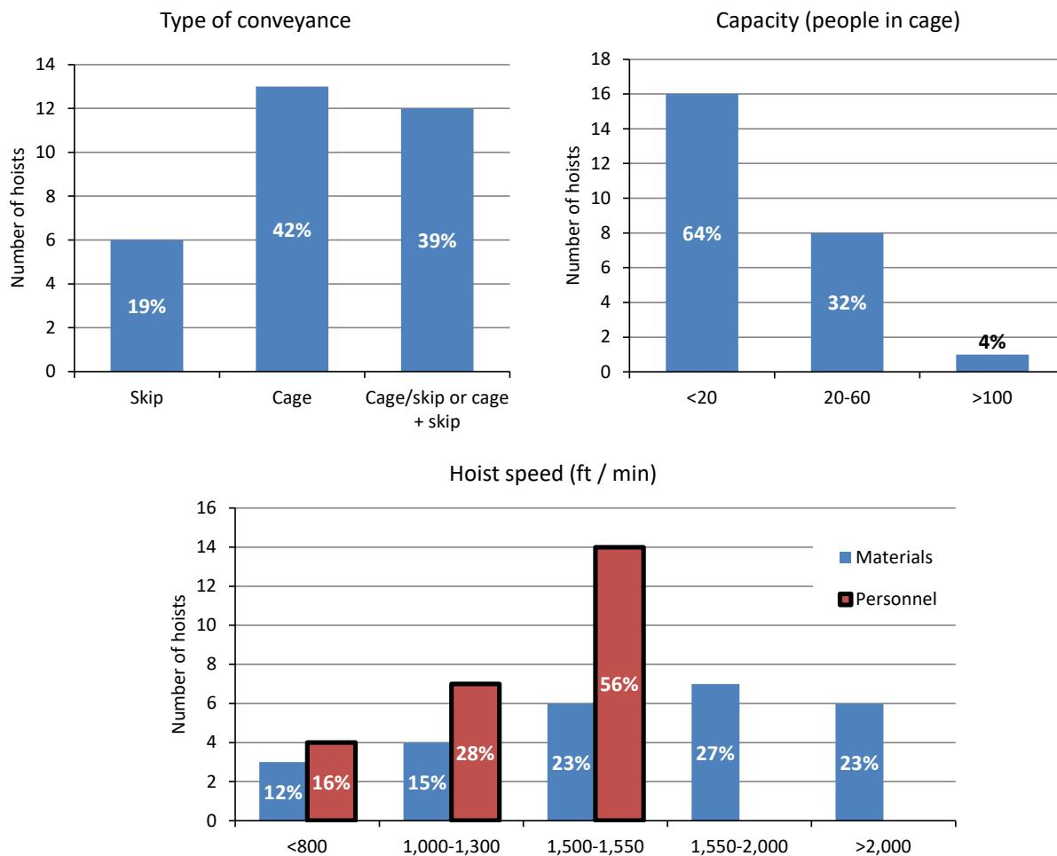
**Figure 4. Type of conveyance, capacity and hoist speed**
