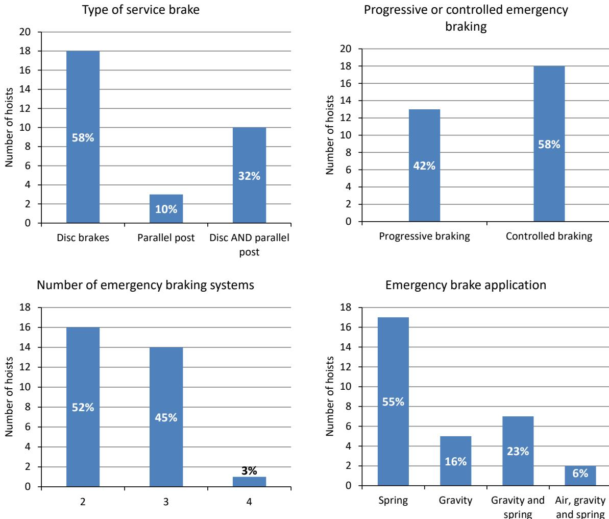
**Figure 6. Braking systems**
