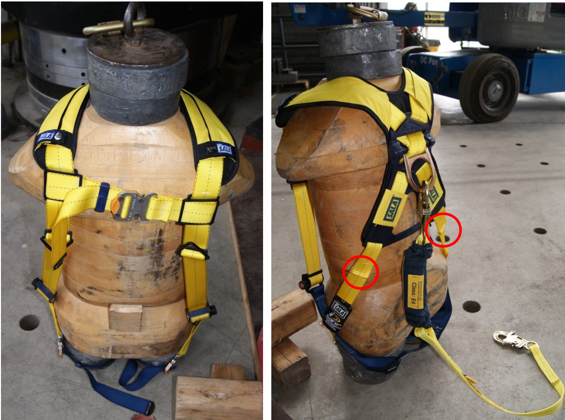
Figure 22 – Wooden torso equipped with a safety harness and a lanyard with a class E4 energy absorber (taken from Leclerc and Tremblay, 2015)
