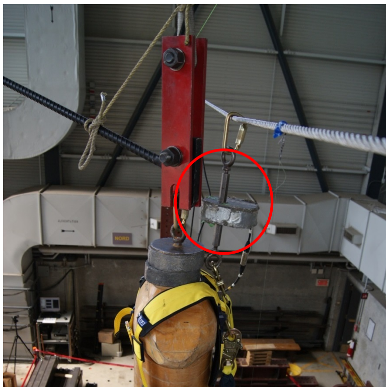
Figure 24 – Load cell (22.3 kN) for measuring lanyard tension (taken from Leclerc and Tremblay, 2015)
