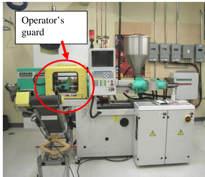
Figure 26 – The studied machine and its operator’s guard [7].
