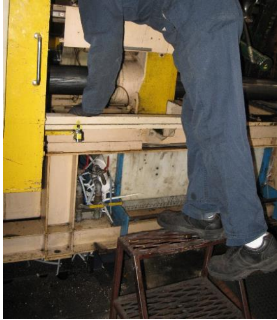
Figure 21 – Worker on a stepladder with narrow steps.
