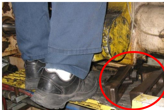
Figure 20 – Worker on a step partially obstructed by clamps.
