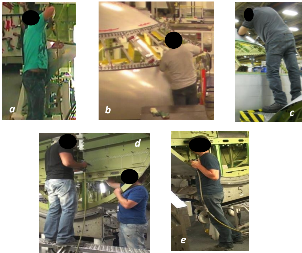
a. and b. Drilling at stations 1 and 2; c. Countersinking at station 2 ; d. and e. A pair of workers and one person alone riveting at station 4.
