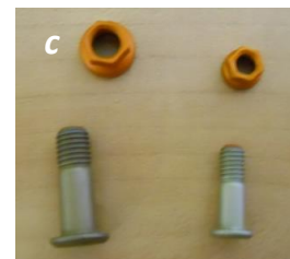
a. Rivets of various sizes; b. Rivets in transparent box used to carry them between workstations; c. Hi-lites (screwed rivets)
