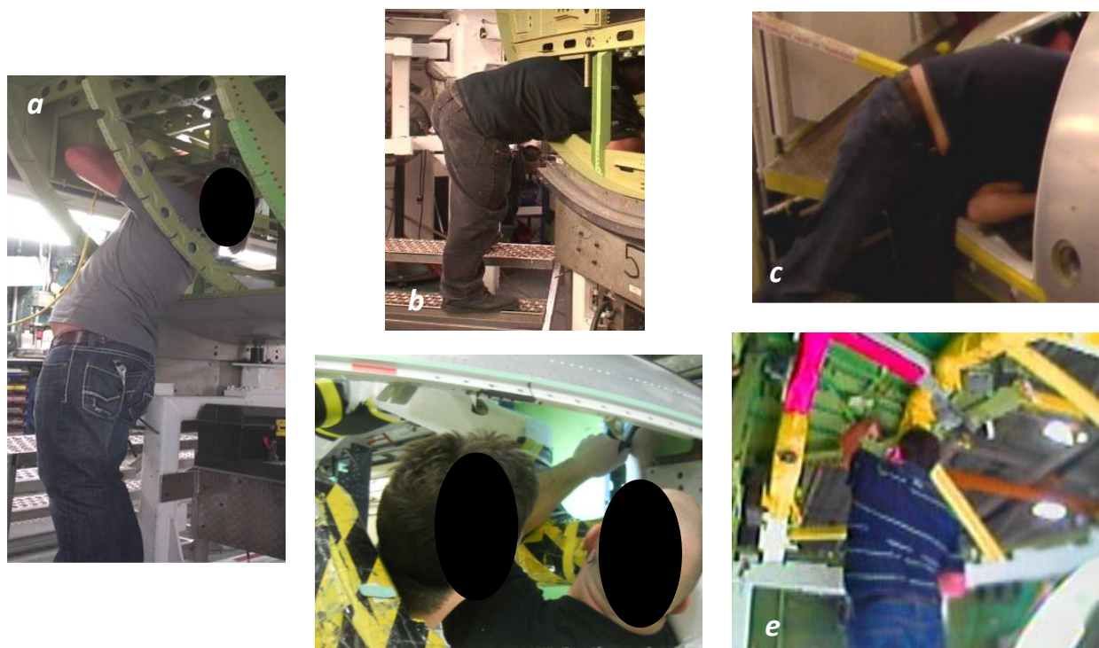
a. b. and c. Cramped spaces involving postural constraints at stations 3 and 4; d. Poor visibility at station 2; e. Demanding work for upper extremities at station 1.
