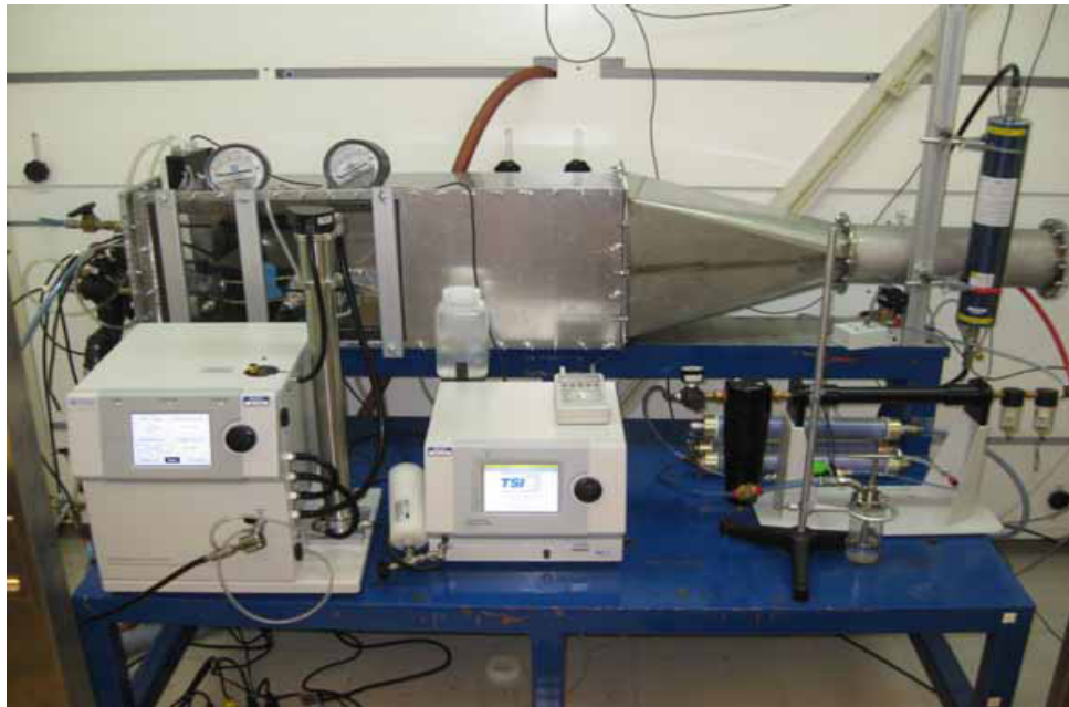
Figure 2.1 – Schematic of the set-up used for evaluating the efficiency of N95 FFRs under constant and cyclic flows [81]
