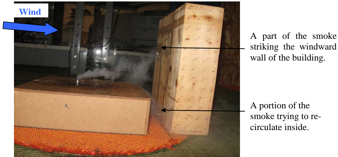
Figure 3.2 – A tall building placed downstream of a low building with source ( \theta = 0^\circ ).
