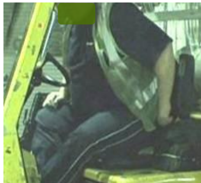
Figure 26. Narrow seat – webbing hard to reach.
