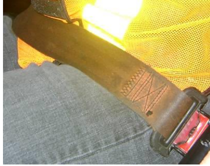
Figure 13. Orange webbing after exposure to a dirty environment.
