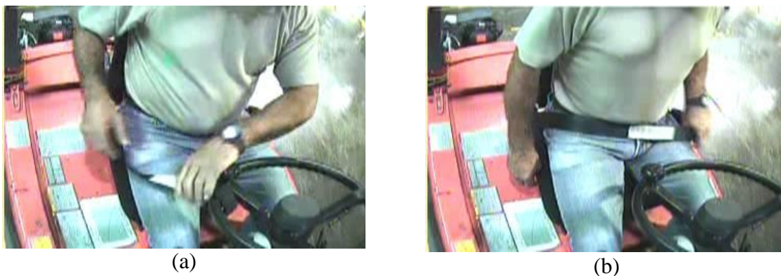
Figure 17. Typical steps in fastening with a manual retractor – without adjustment.
