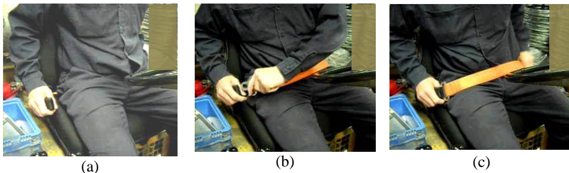
Figure 15. Fastening when the buckle is not rigidly fixed (ALR).
