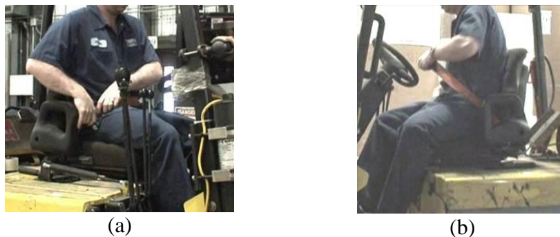
Figure 18. Typical steps in unfastening an ALR or ELR seat belt.
