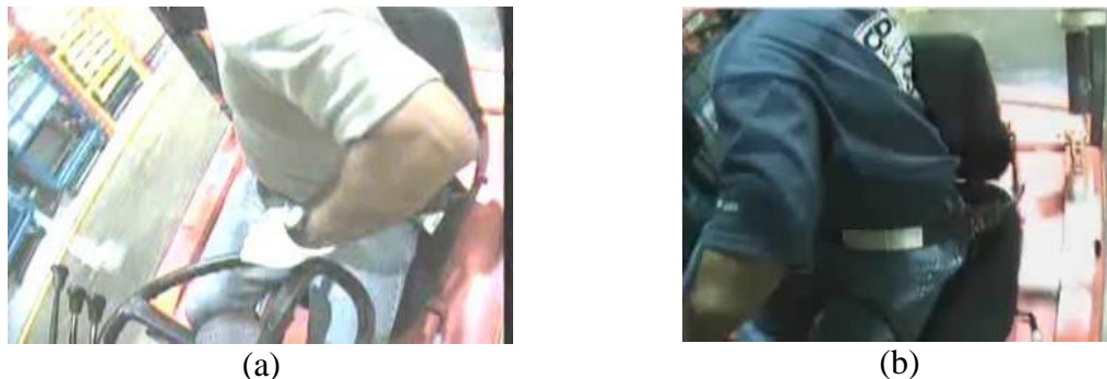
Figure 33. Manual retractor – turning around to see while reversing.
