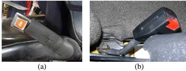
Figure 30. Types of buckle buttons.
