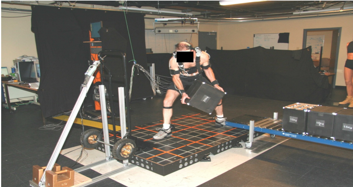
Figure 2.2 Experimental setup for the 90° condition. The subject is moving the box from the conveyor to the hand trolley.
