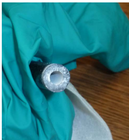
Figure 7 – Photograph of SMPS pipe intake after attempt to detect TiO 2 powder NPs
