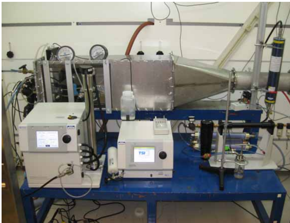
Figure 2-3: Schematic of the test system used to challenge N95 respirators against poly-dispersed aerosols.
