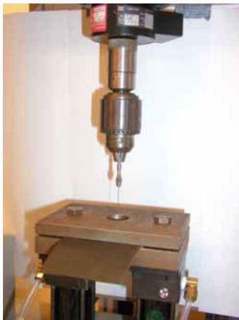
Figure 6 – Setup for needle puncture measurement
