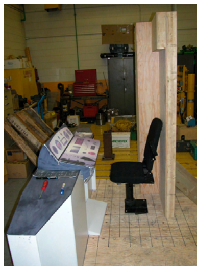
Simulations on a full-scale model of an operator cab.
