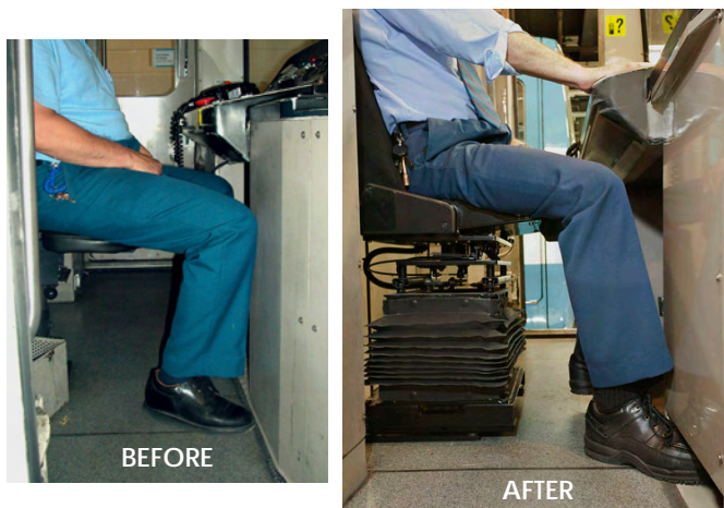
Improved positioning of the right leg due to the modifications made to the control console in the cab.
