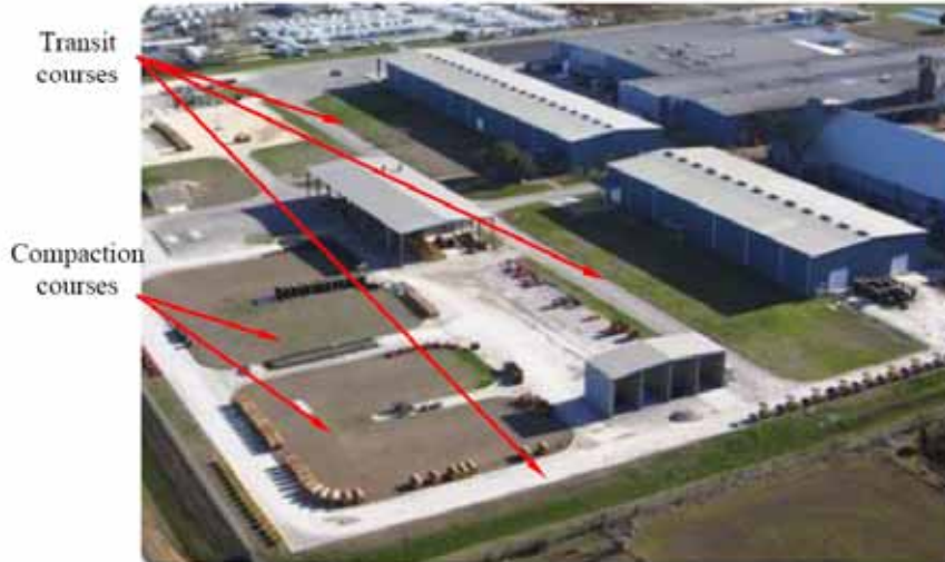
Figure 3.1: View of the test track used for measurements during compaction and transit modes.
