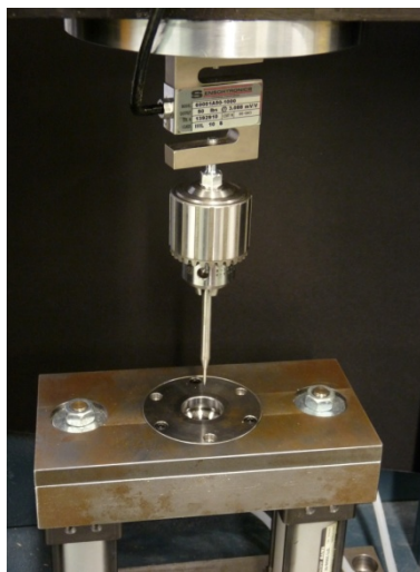
Figure 4 - Photo du montage de perforation
