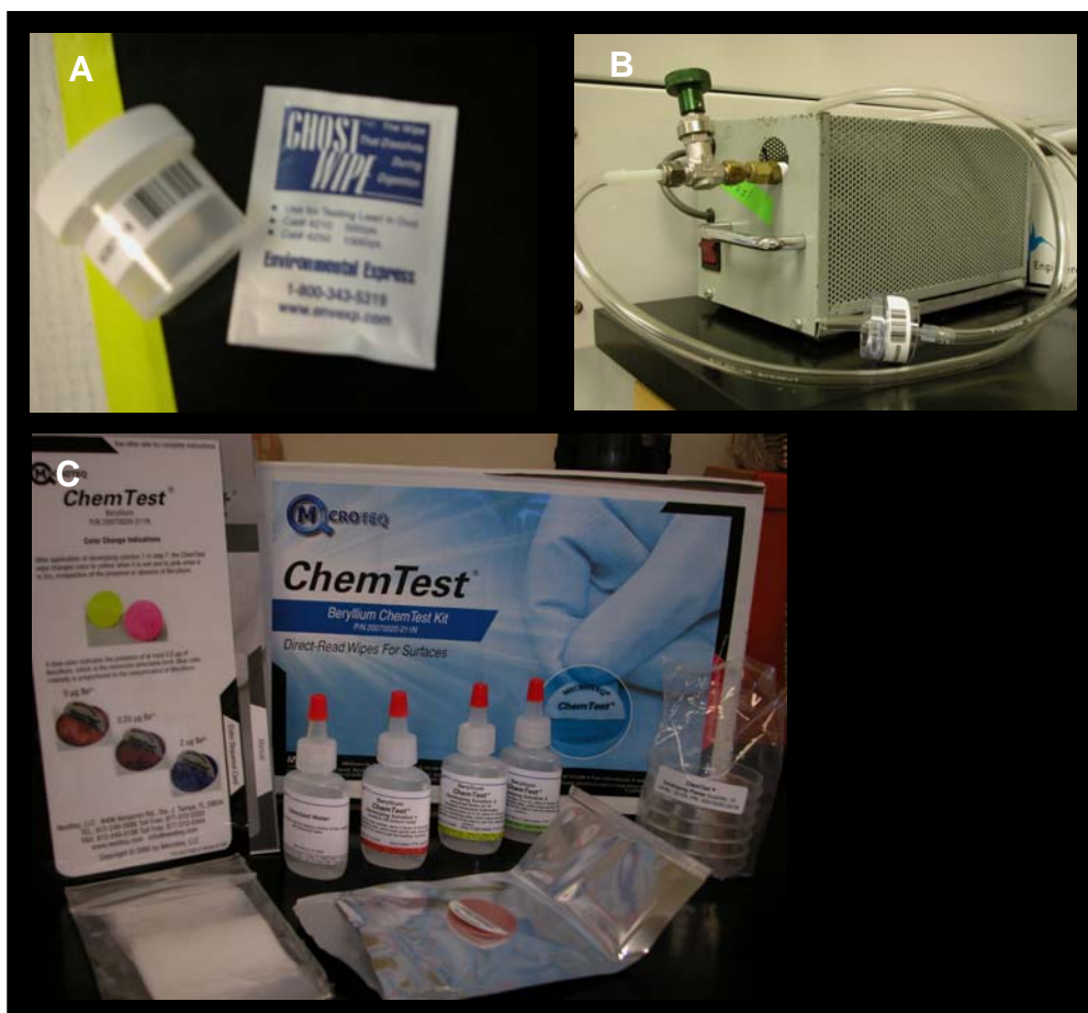
Figure 6 : Techniques d'échantillonnage . A – lingettes humides (Ghost Wipe®), B – aspiration (micro-vacuum), C – colorimétrie (ChemTest®)
