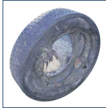
Photo no. 2: Tire that burst, semi-trailer hit by an electric arc near a high voltage line.
