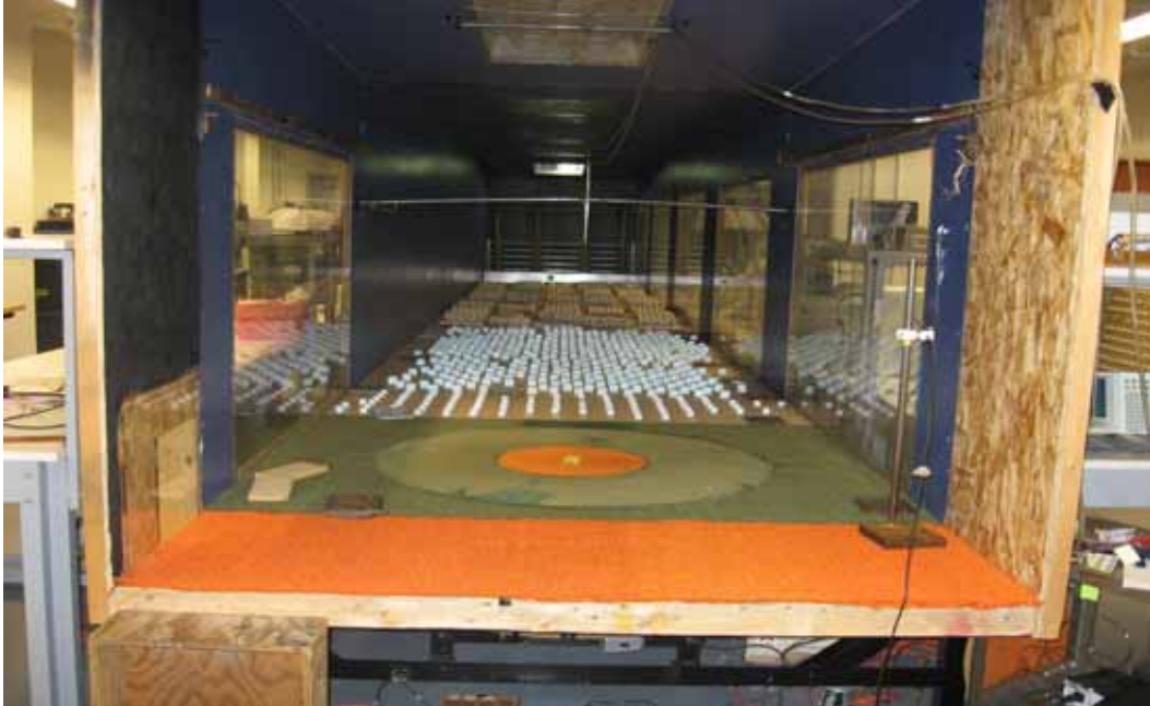
Figure 4.1 Front view section of the Boundary Layer Wind tunnel at Concordia University.
