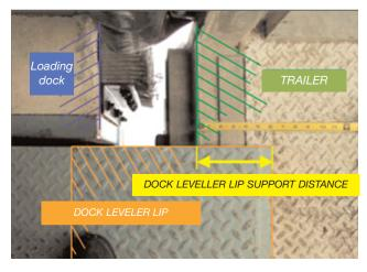
The lip support distance represents the possible advance distance for the trailer without the lip tipping and creating a dangerous space between the loading dock and the trailer.
