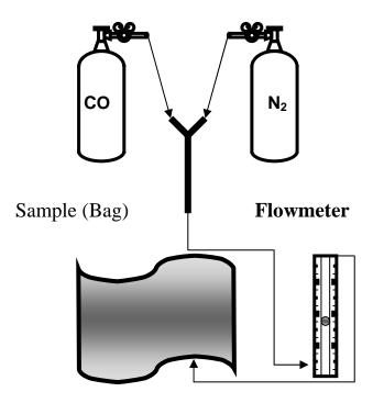
Figure 5. Preparation of  $CO/N_2$  gas mixture
