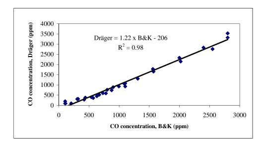
Figure 8. Comparison Dräger vs.  $B\&K - CO/N_2$  mixture
