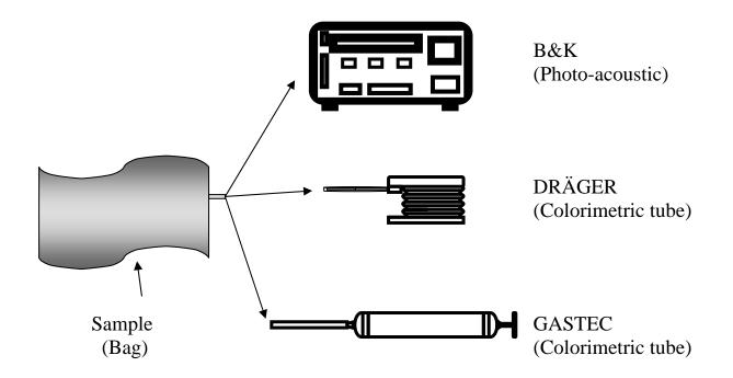
Figure 6. Carbon monoxide sample collected in a bag
