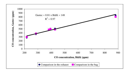
Figure 11. Comparison Gastec vs. B&K - Diesel test bench
