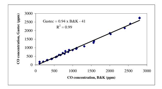
Figure 9. Comparison Gastec vs.  $B\&K - CO/N_2$  mixture
