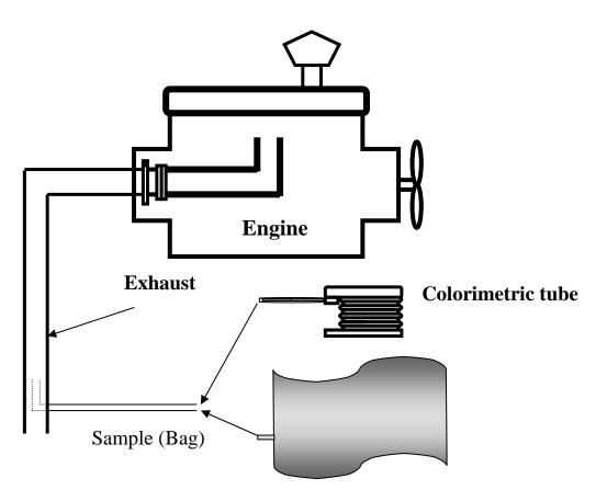
Figure 7. Evaluation instrumentation on a diesel test bench
