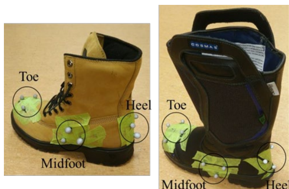
Figure 20. Motion capture markers attached to footwear F1 (left) and F5 (right).
