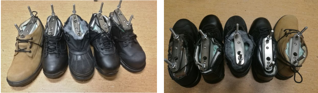
Figure 11. Boot laces and stuffing used to keep the lasts from shifting inside the boots.
