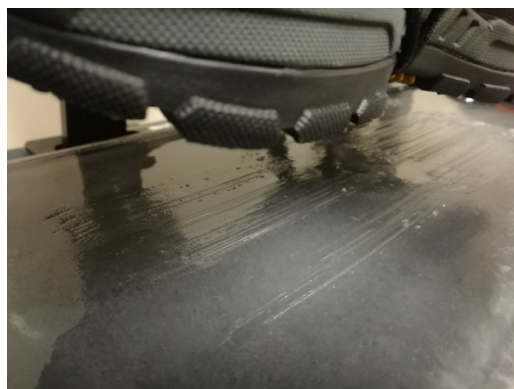
Figure 9. Deep scratches made by F9 sole (having the Green Diamond technology) on wet ice.
