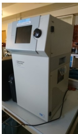
Figure 2. Engine exhaust particle sizer (EEPS).
