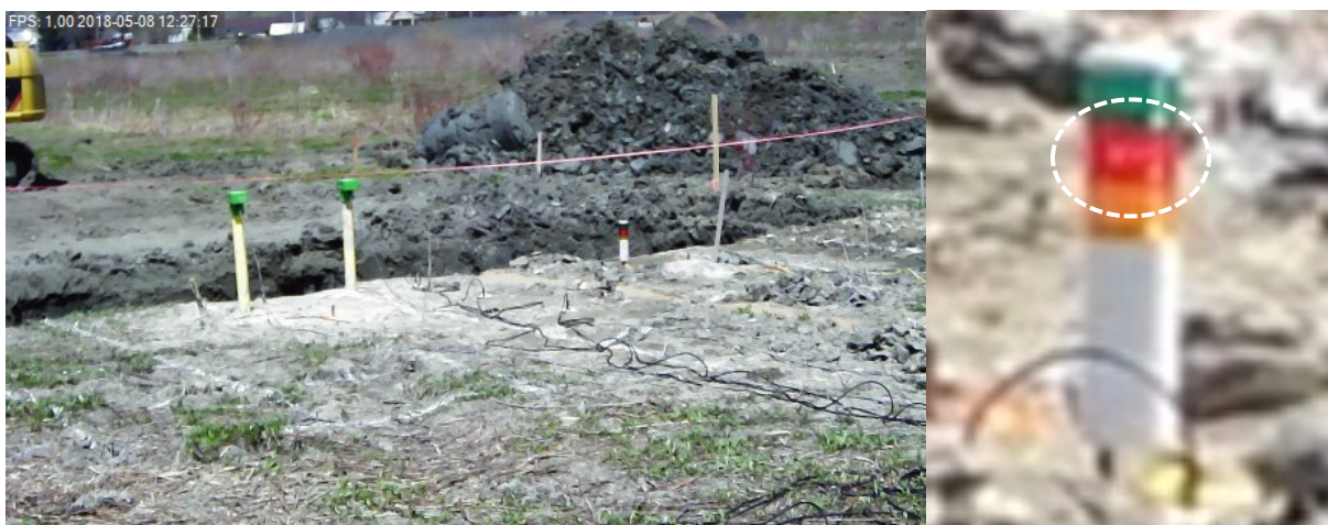
Figure 36. Flashing red light of D2 warning, following the detection of the third creep phenomenon prior to failure.
