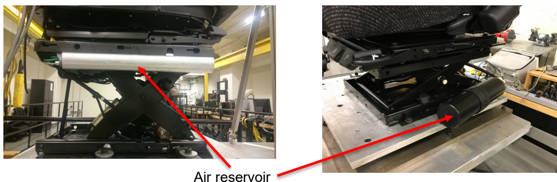
Figure 4.6. Pictorial views of suspension mechanisms with an additional air reservoir.
