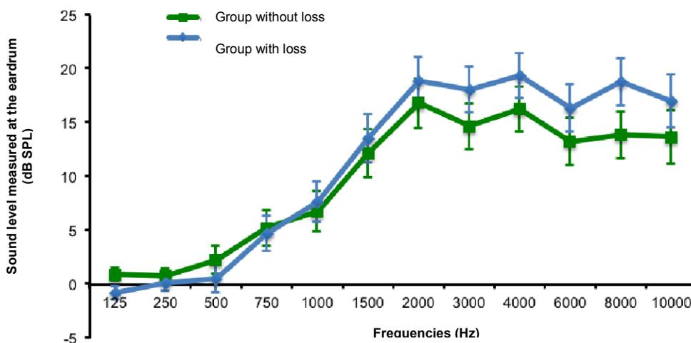
**Figure 11. Mean of the stimulation levels measured at the eardrum according to frequency (standard error of the mean) for each of the groups**
