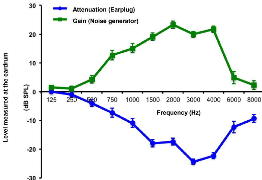
**Figure 2.** Mean of attenuation levels (standard error of the mean) of earplugs (green) and stimulation from noise generators (blue) according to frequency
