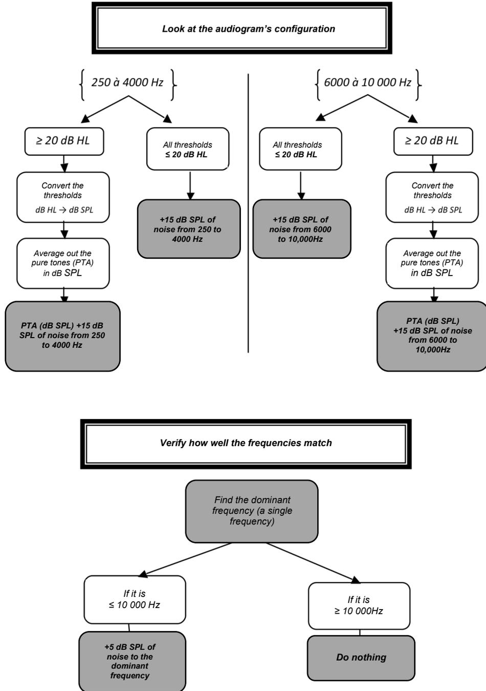
Figure 10. Algorithm to adjust noise generators in Study 2
