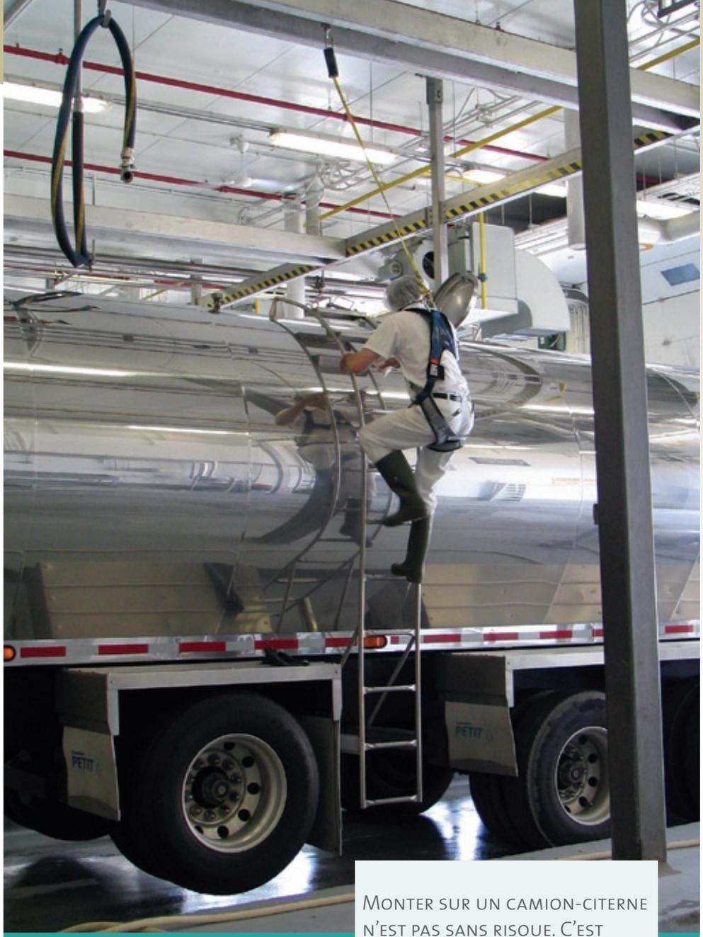
MONTER SUR UN CAMION-CITERNE N'EST PAS SANS RISQUE. C'EST POURQUOI UN DISPOSITIF D'ANCRAGE PERMANENT A ÉTÉ INSTALLÉ. LES TRAVAILLEURS S'Y ATTACHENT AVANT DE GRIMPER.
