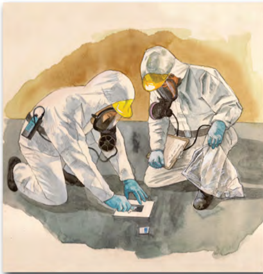
Figure 4: Wipe sampling with a moistened wipe
