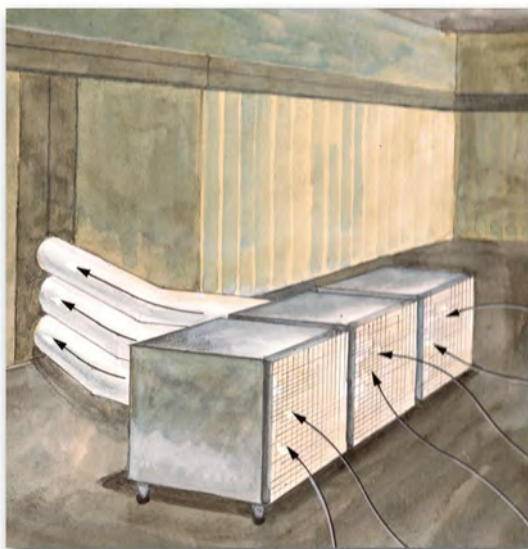
Figure 7: Negative pressure system
