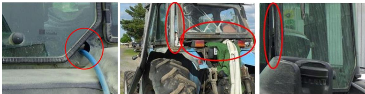
Figure 10. Non-airtight tractor cabs observed
