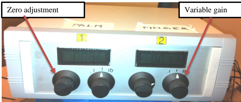
Figure 3.3 A two-channel signal conditioner developed for simultaneous acquisition of finger- and palm-side FlexiForce ® sensors.
