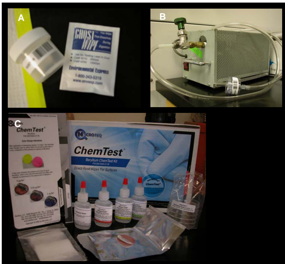
Figure 6: Sampling techniques . A – moistened wipes (Ghost Wipes ® ), B – micro-vacuuming, C – colorimetry (ChemTest ® )
