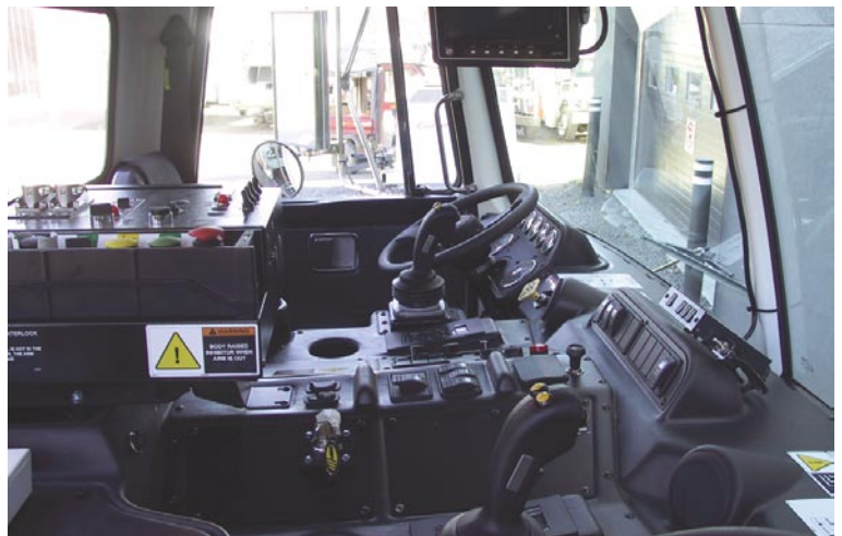
PHOTO 1 ADJUSTABLE CONTROL LEVER AND STEERING WHEEL AT AN ANGLE OF 15°
