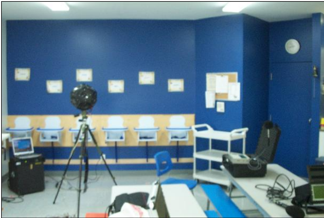
Figure 4 Spherical noise source for measuring reverberation time at location 1 in day-care centre C)
