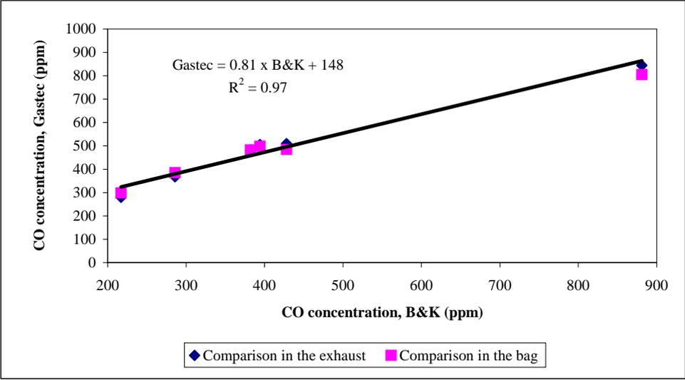
Figure 11. Comparison Gastec vs. B&K – Diesel test bench
