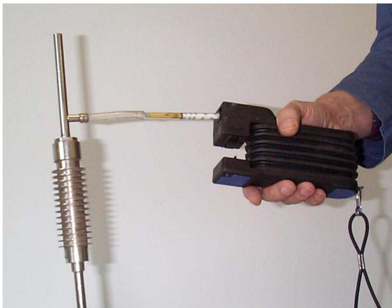
Figure 3. Dräger sampling probe for high-temperature application
