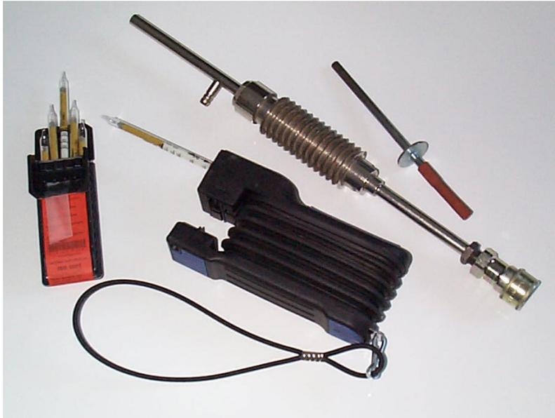
Figure 2. Dräger sampling system, carbon monoxide measurement
