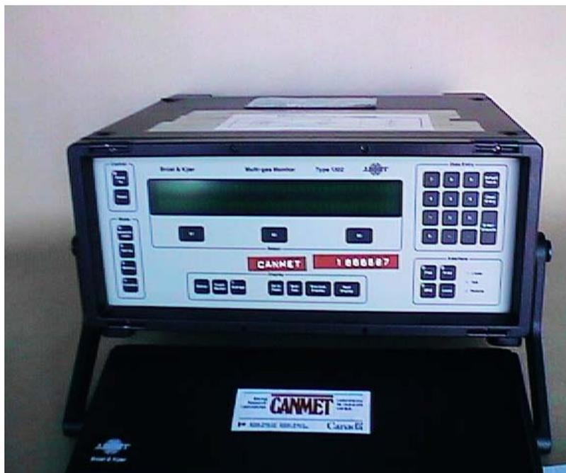
Figure 4. B&K photo-acoustic gas sampler (model 1302)
