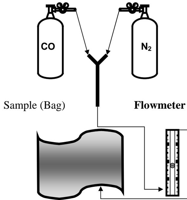
Figure 5. Preparation of CO/N<sub>2</sub> gas mixture
