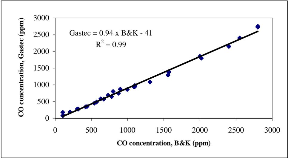
Figure 9. Comparison Gastec vs. B&K – CO/N<sub>2</sub> mixture
