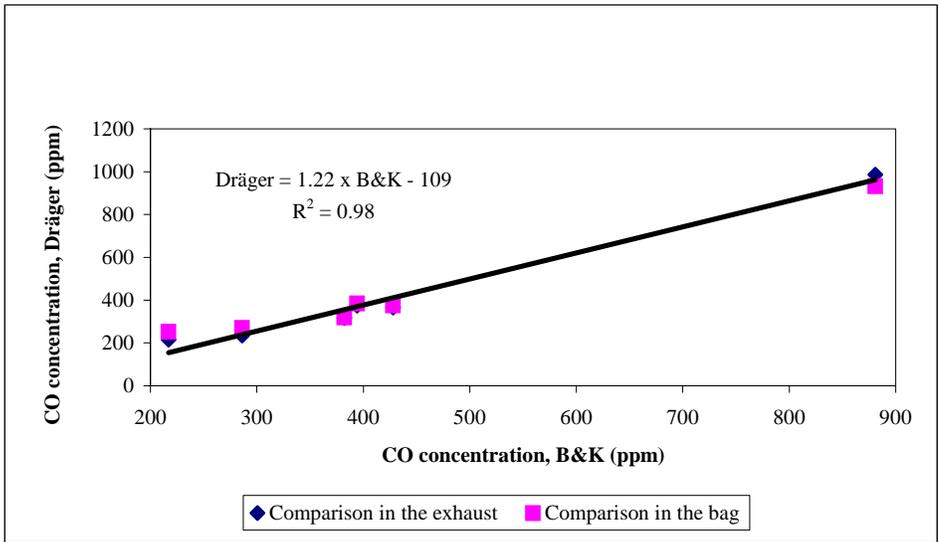
Figure 10. Comparison Dräger vs. B&K – Diesel test bench
