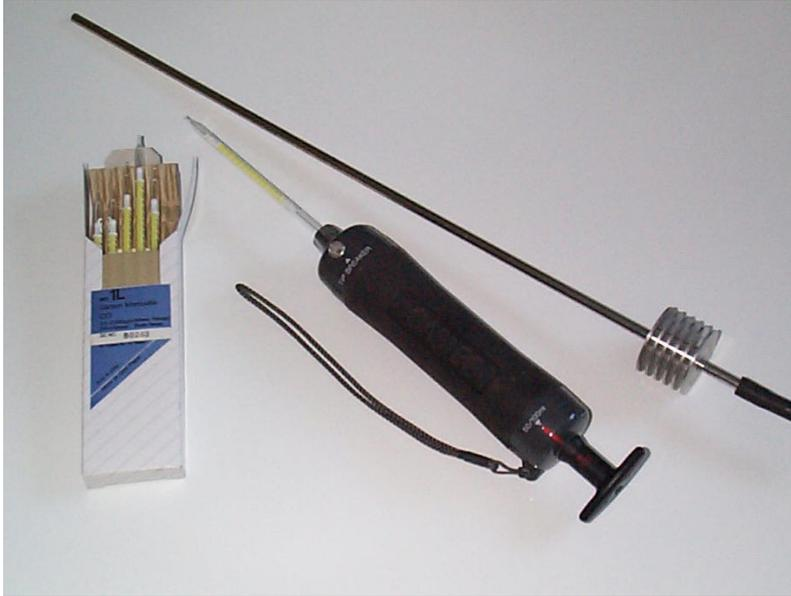
Figure 1. Gastec sampling system, carbon monoxide measurement
