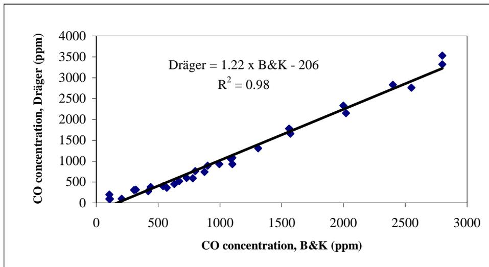
Figure 8. Comparison Dräger vs. B&K – CO/N<sub>2</sub> mixture
