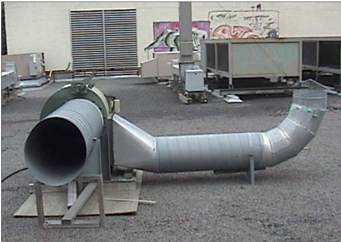
Figure 4.8 Photograph of the test stack used on the BE building (low stack with h_s=1\text{m} )
