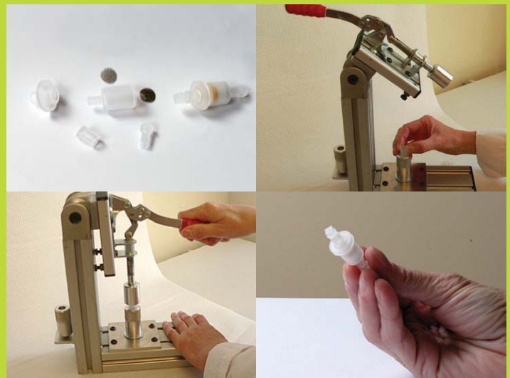
Assembling the cassettes needed for nitrosamine analysis previously required repetitive fine-motor manipulations and the exertion of force. Thanks to the above device, which was developed in the IRSST's laboratories, these gestures are no longer necessary.
